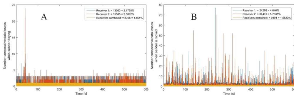
**Figure 1 A,B:** Loss of wireless transmitted real-time data in consecutive time frames. Data loss varies based on the data recorded from receiver 1, receiver 2, or the combined signals of both receivers. Data was recorded in real-time at a data rate of
